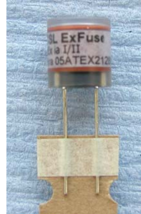
Body D:10mm x L:11mm Lead Length 16mm Lead Pitch 5.08mm
